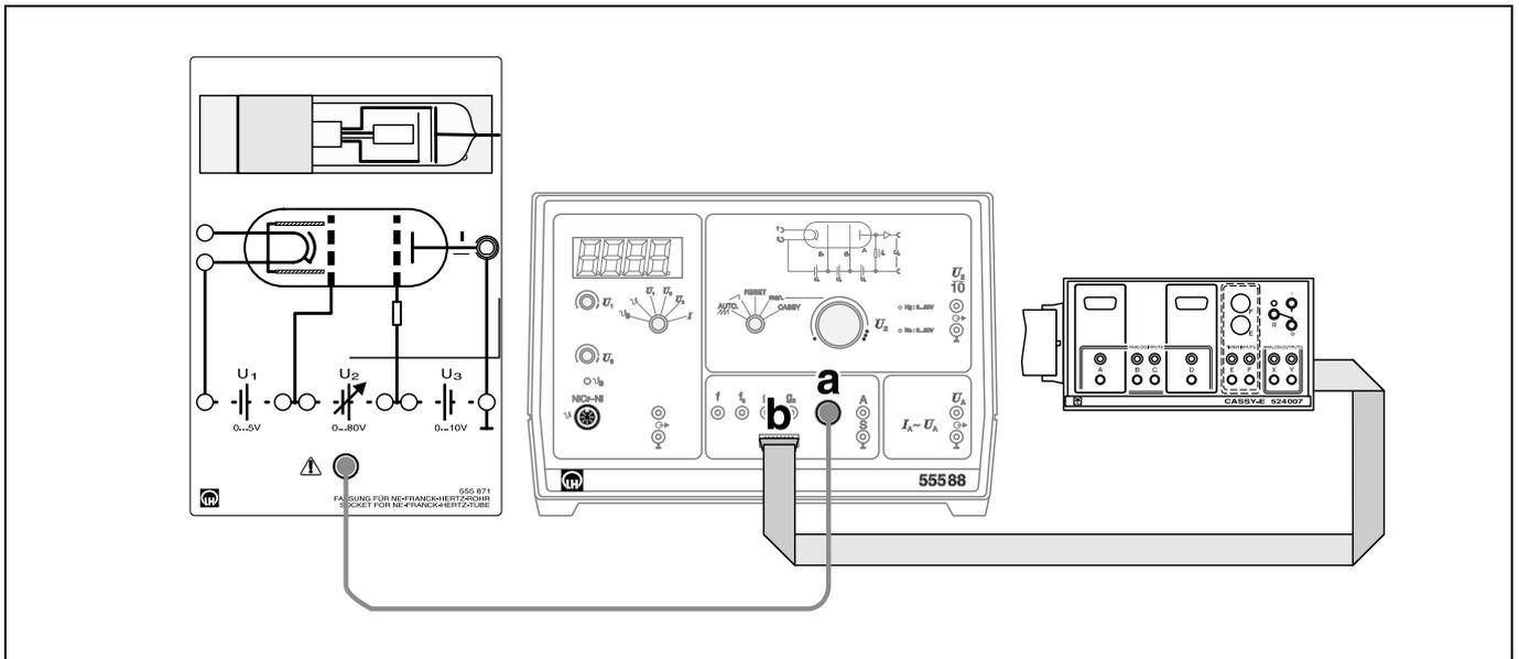
Fig. 2: Experiment setup for Franck-Hertz experiment for neon
