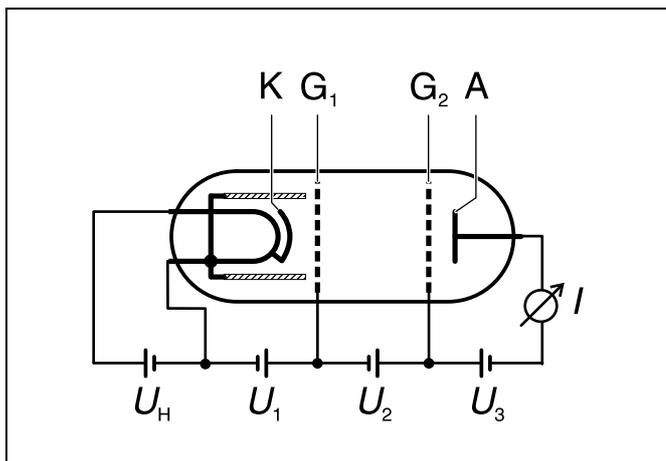
As the acceleration voltage  $U_2$  increases, the electrons attain the energy level required for exciting the neon atoms at ever greater distances from grid  $G_2$ . After collision, they are accelerated once more and, when the acceleration voltage is sufficient, again absorb so much energy from the electrical field that they can excite a neon atom. The result is a second maximum, and at greater voltages  $U_2$  further maxima of the collector currents  $I_A$ .
