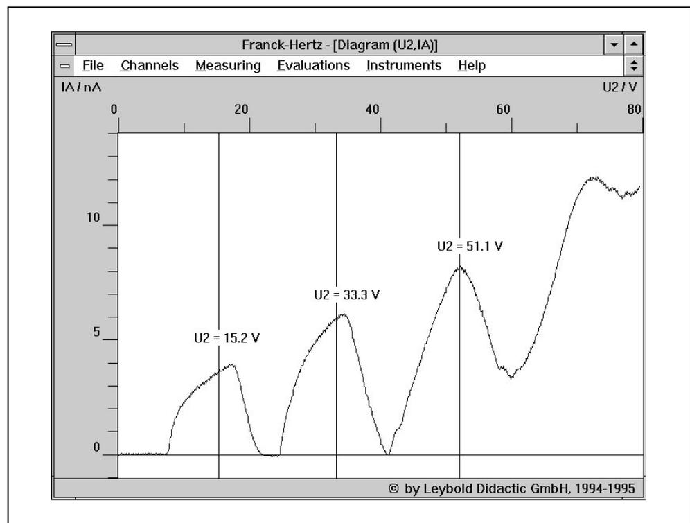
Fig. 4: Franck-Hertz curve for neon (recorded using an XY-recorder)
